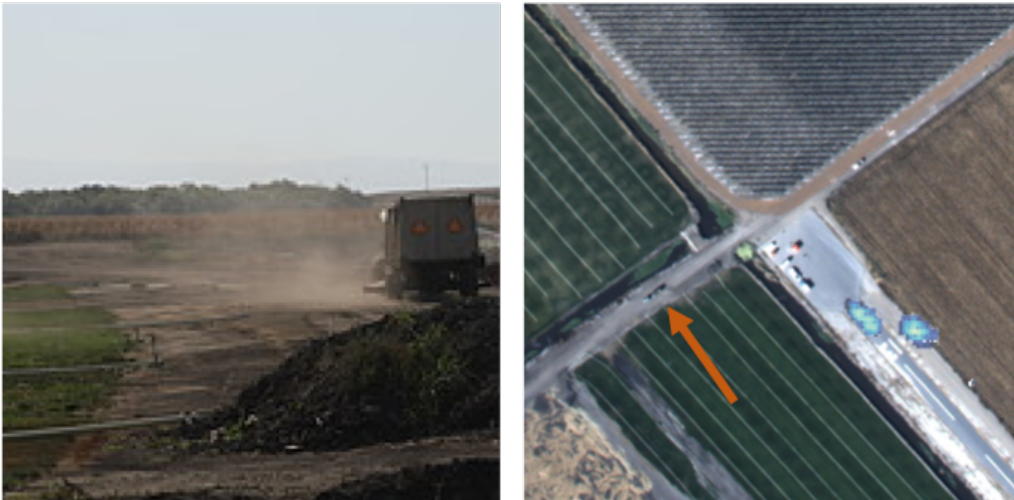
Figure 6: Dust clouds created by equipment (left) create no detectable interference to the methane signal produced by LeakSurveyor instrumentation (right, no methane signal observable at dust cloud, orange arrow). Methane signal is clearly observable over the release site (right).
