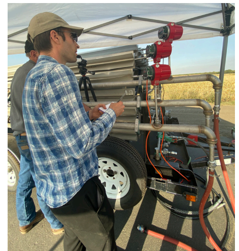
Evan Sherwin calibrates natural gas flow meters at the pressure and temperature regulator trailer, through which we released gas from pressurized trucks, with help from technician Jeff Gamble of Rawhide Leasing. The three-meter setup allows us to maintain reliable measurements at a wide range of gas release volumes.
